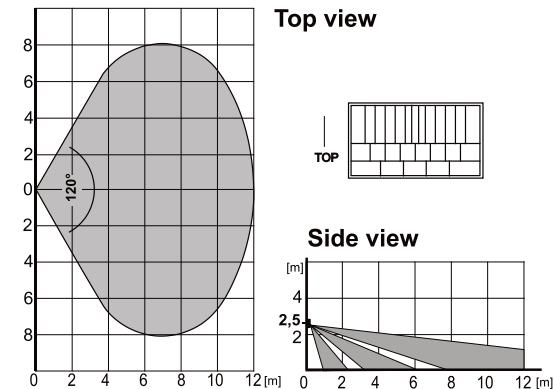
The characteristics can be changed by using optional lenses:
