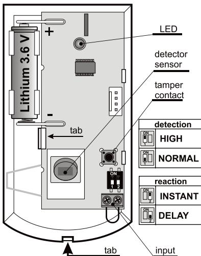
1. Open the detector cover by pressing the tab. Avoid touching the internal PIR element or damaging the antenna.
